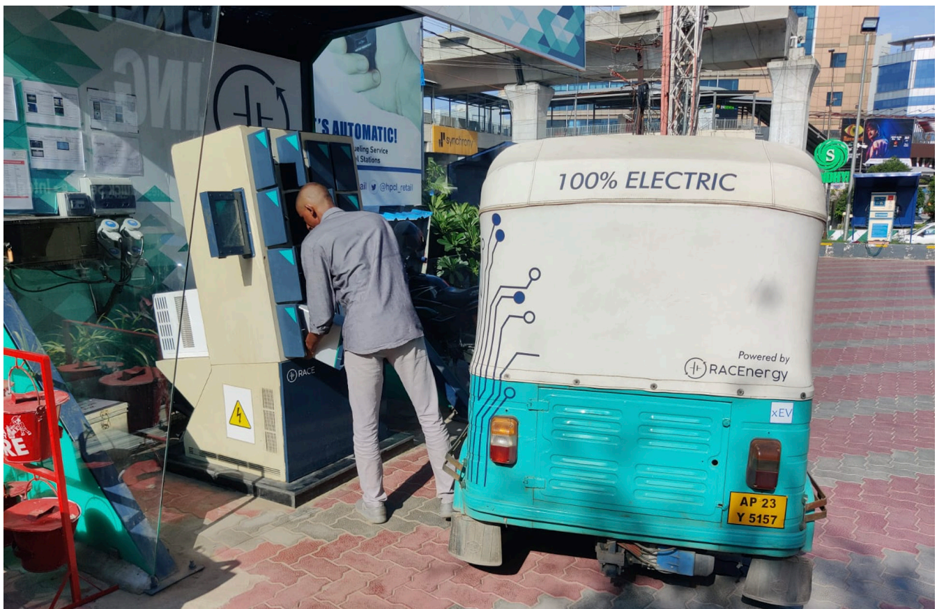
FIGURE 14 | An e-3W battery-swapping station in Hyderabad
